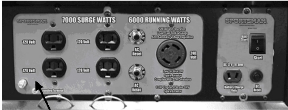
Figure 3 - Attaching the Grounding Wire to this Generator
