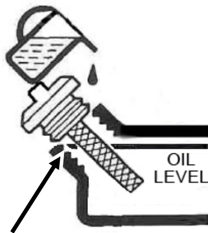
Figure 2 - Add Oil To TOP Of Threads
